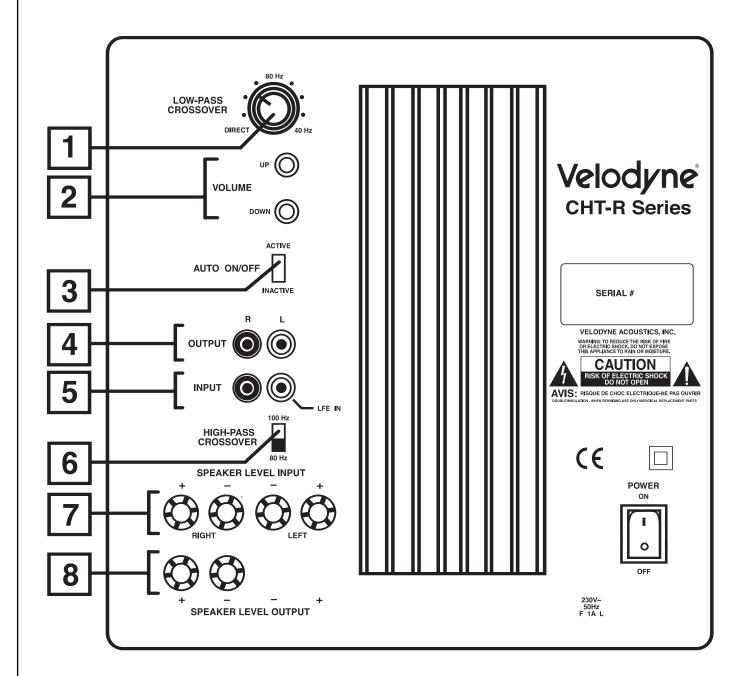
Figure 1. CHT-R Rear Panel Connections
